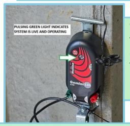
7. Plug transformer into the wall socket and turn on. The upper section of the controller should now have a pulsing green light and the outside red warning light will also pulse indicating that the system is now 'live'!
