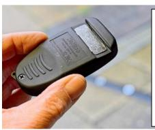
4. Using the tester (LED's uppermost and metal strip on underside resting on top fence wire) press and hold down the main central red button to ensure fence is now deactivated - No LED's illuminating
